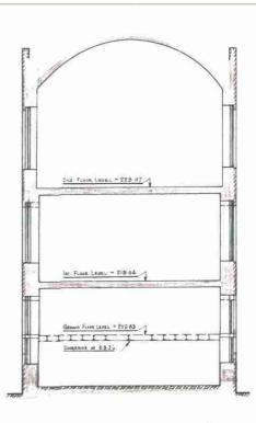
Figure 15. 15.1, left, section through the Worthington wing c.1970, showing original stack levels. 15.2, right, section through the Jackson wing c.1970 showing the original floor heights and the projected level of the extant ground floor
