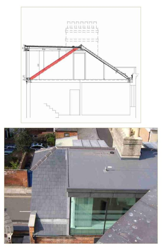
Figure 6. 6.1, top, post 2003 section (running east to west) of the attic of 2-4 St. John Street. The dormer extension can be seen on the left-hand side of the image. 6.2, bottom, the 2003 dormer at the rear of 2-4 St. John Street from the Sackler
