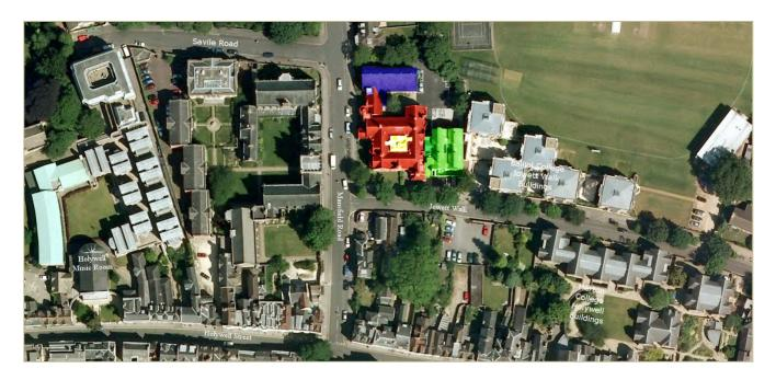
Figure 1. Map showing 3 Mansfield Road and the surrounding area, orientated with North at the top of the image. The original portion of the building is highlighted in red, the 1965-68 library extension is highlighted in blue, the 1987-88 courtyard infill is highlighted in yellow, and the 2007-9 extension is highlighted in green
