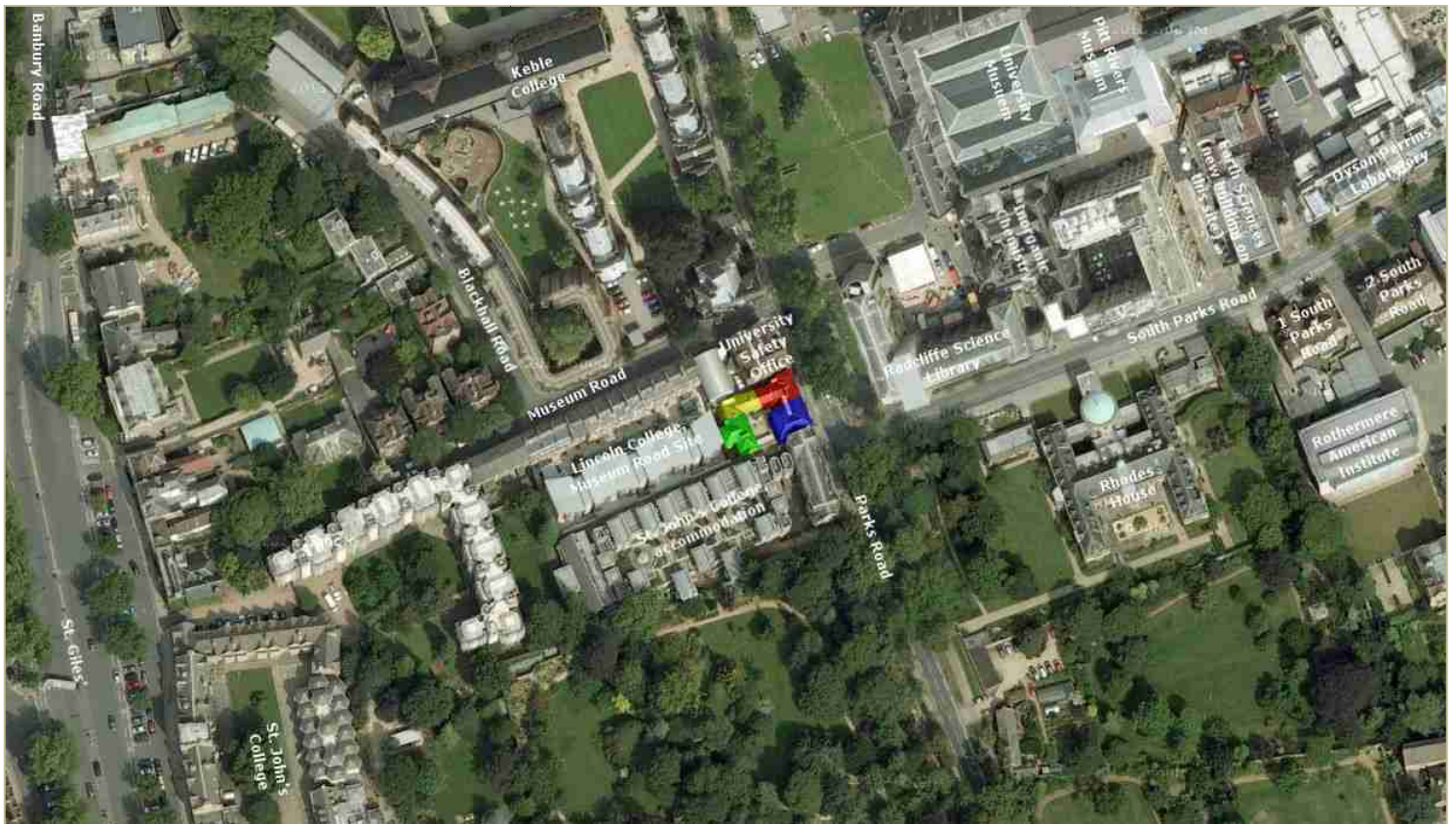
Figure 1. Satellite image of 9 Parks Road and the surrounding area. The original portion of the building is highlighted in red. The 1925 extension is highlighted in blue, the 1932 extension is highlighted in yellow, and the 1938 extension is highlighted in green
