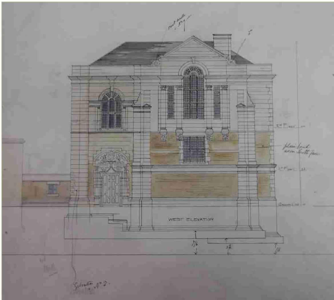
**Figure 13. Jackson's original plan for the western elevation of the Radcliffe Science Library. Note, the elaborate doorway on the left-hand side of the image (on the western elevation of the eastern cross-wing), was replaced with the extant window into the stair lobby in 1933-4. The corridor on the left-hand side of the image, leading to the Abbot's Kitchen, was provided with a first-floor addition in the 1950s or 60s**
