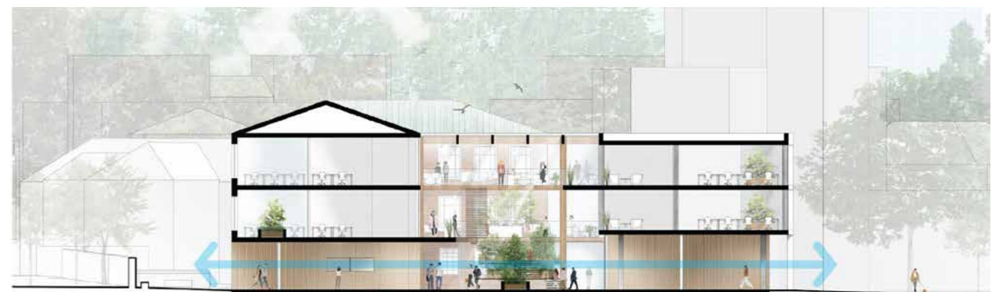
Illustrative concept section through building showing link from ROQ through to the external garden
